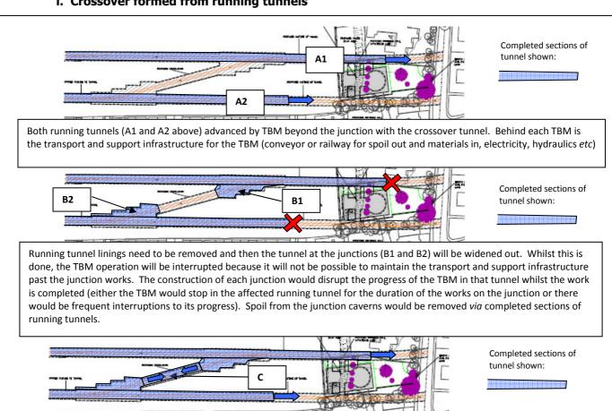
resume without further interruption. The crossover itself (C) can be completed between the junction caverns whilst the TBM is operating (from one end or the other or in both directions alternately or simultaneously).
