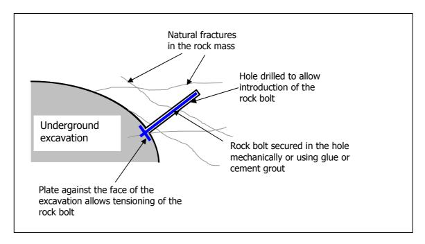
There are many different types of rock bolt and different methods for fixing them; the choice of bolt in a given situation depends upon a detailed assessment of the ground conditions and the nature of support needed. The key features of their installation is that a hole must be drilled to
